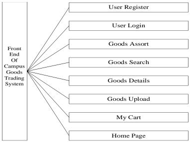
Figure 1 Front-end function module diagram of the system
